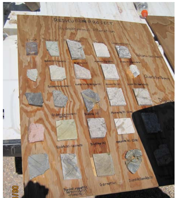
This helpful display shows the various types of alteration seen in the different rock types at the deposit.
