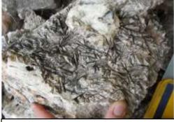
Figure 3: Banded, gold-bearing, quartz-calcite-adularia vein and details of encrust-
