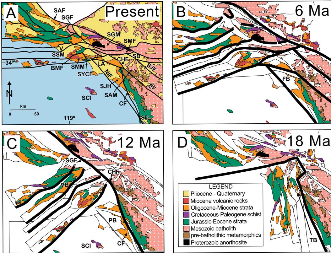
Figure 1. Present and palin-spastic geologic maps of Los Angeles area. Legend in D is for A-D. In B-D, light lines (some of which are known or suspected faults) separate blocks used in palin-spastic reconstruction; heavy lines are presumed active faults. See Ingersoll and Rumelhart (1999) for detailed caption. See Figure 2 for location.
