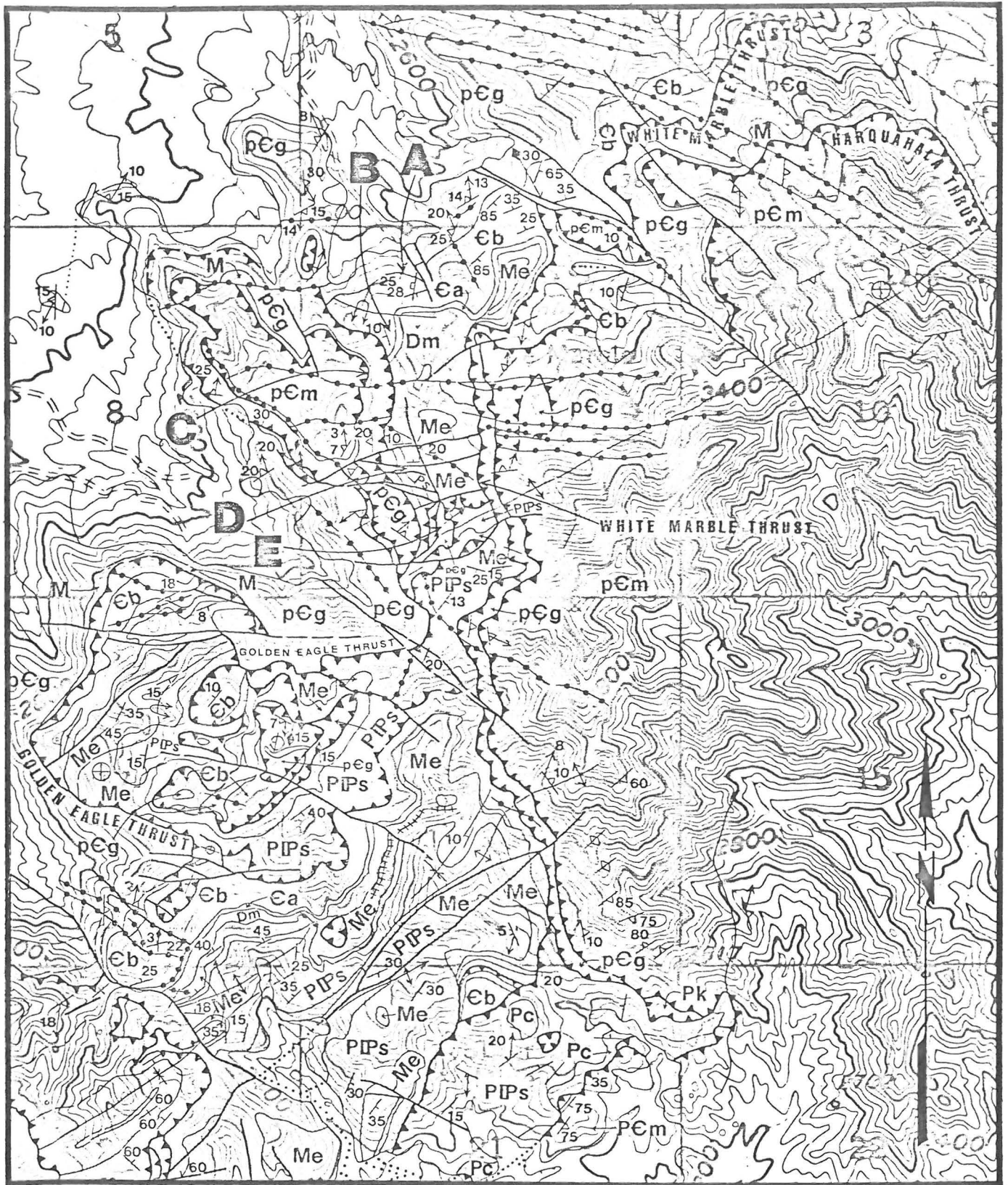
Figure 7. Geological map of White Marble mine and vicinity. Symbols are as follows: pEg = mylonitic porphyritic granite (protolith equals probable 1400 m.y. biotite granite) and minor amounts of probable Precambrian alaskitic granitoids; Eb = Cambrian Bolsa Quartzite; Ea = Cambrian Abrigo Formation; Dm = Devonian Martin Formation; Me = Mississippian Escabrosa Limestone; PPs = Permian-Pennsylvanian Supai Formation; Pc = Permian Coconino Sandstone; Pk = Permian Kaibab Formation; M = ultramylonite at Harquahala thrust. Diamond-shaped arrows are slickensides; arrows are lineation on foliation surfaces. pEm = Precambrian age amphibolite grade metavolcanic and metasedimentary rocks locally intruded by probably Precambrian age alaskitic rocks.
