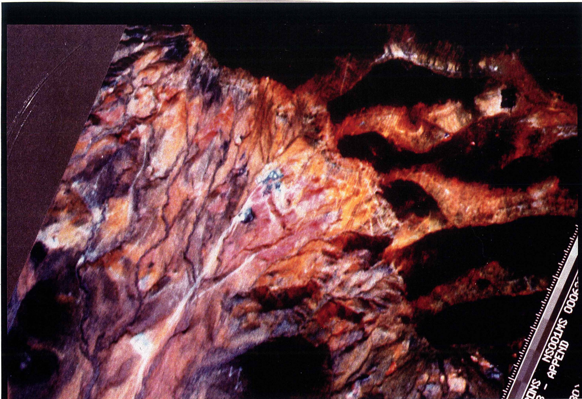
Figure 12. Simulated Thematic Mapper image of the Kennecott area at 1:24,000 scale. This is a canonical transform image processed by the Jet Propulsion Laboratory from NASA NS-001 airborne scanner data (courtesy of the Geosat Committee, Inc.).
