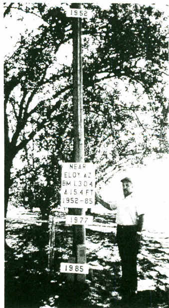
Figure 5. The land subsided more than 15 feet in Pinal County south of Eloy from 1950 to 1985. The marker on the pole shows where the land surface was in 1952. More subsidence has undoubtedly taken place since 1985. Photograph provided by H.H. Schumann.
